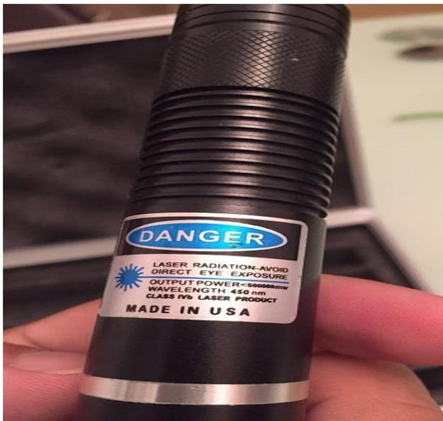
**Figure 1:** Class IVb blue laser pointer with a 50000 mw output power and 450 nm wave length
