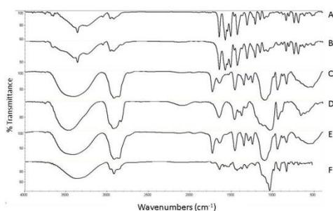
**Figure 3:** Fourier transform infrared spectrum of (A) atorvastatin, (B) atorvastatin + hydroxypropyl methylcellulose, (C) atorvastatin-loaded nanoemulsion-based film, (D) hydroxypropyl methylcellulose, (E) plain film (not loaded with ATC), and (F) control film (without nanoemulsion base).
