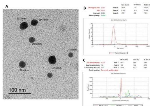
**Figure 2:** (A) Transmission electron micrograph of atorvastatin calcium-loaded nanoemulsion (NE2) showing size and morphology of oil droplets. (B) Particle size and particle size distribution of NE2. (C) Zeta potential of NE2.
