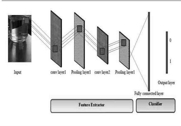
**Figure 5** Architecture of the Convolutional Neural Network.
