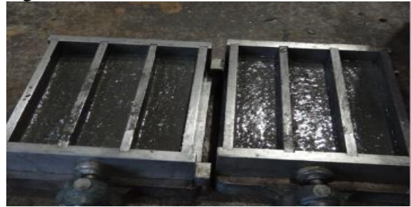
Figure 3 ECC specimens (2cm thick)
