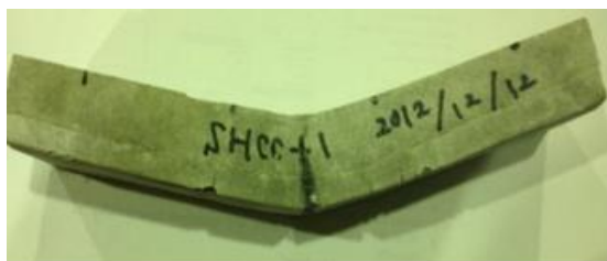
Figure 14 Deformed and cracked SHCC specimen under impact loading
