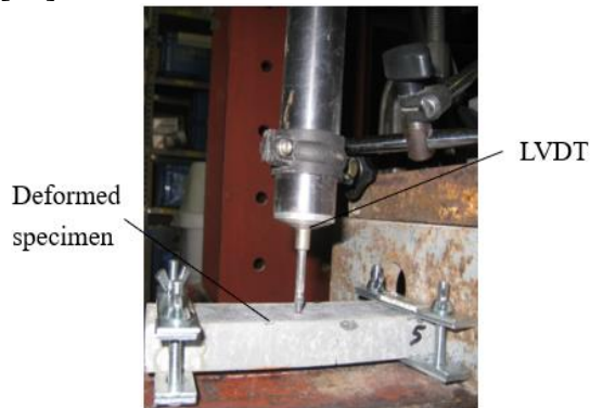
Figure 4 Measuring deflection using LVDT
