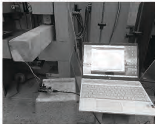
Figure 4 Test setup for measuring the acceleration of a concrete beam specimen
