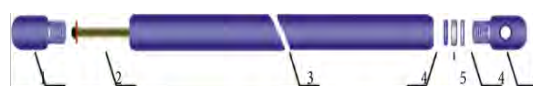
Figure 3 Structure of CO 2 cracker. Key: 1 - Filling valve; 2 - Heating pipe; 3 - Main pipe; 4 - Sealing gasket; 5 - Shearing piece; 6 - Energy release head.
