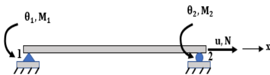
Figure 2 Basic forces of 2D beam-column element
