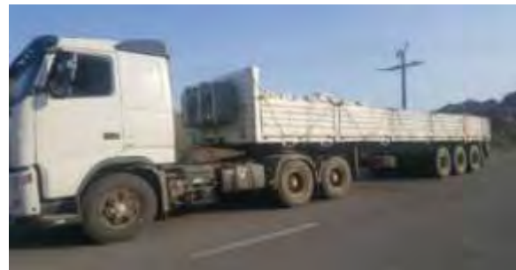
Figure 11 Truck used for loading test
