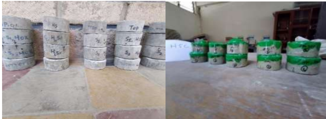
Figure 2. Sorptivity test specimens after cutting cylinder.
