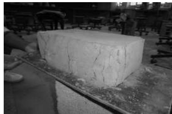
Figure 4: Failure pattern of adobe brick at the end of compression test
