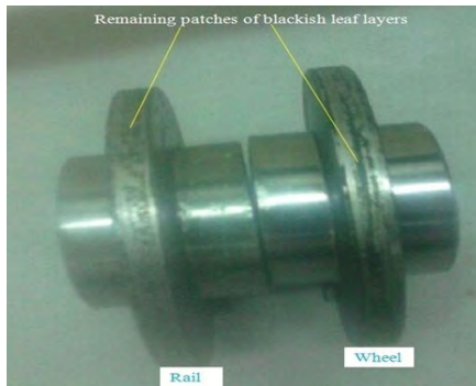
Figure 11 Rail and Wheel discs after leaf test with blackish leaf layers
