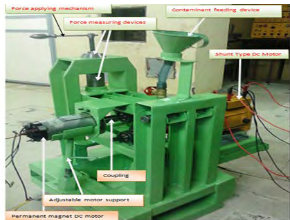
Figure 6 Constructed Twin disc Machine
