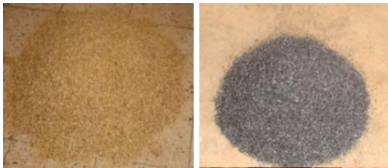
Fig. 3.2: Sample rice husk and its carbonaceous char residue
