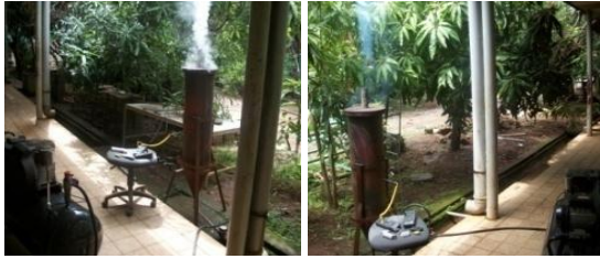
Fig. 3.1: Color change of smoke during the carbonization process
