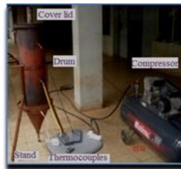
Fig. 2.2: Experimental Setup for Carbonization of Rice Husk
