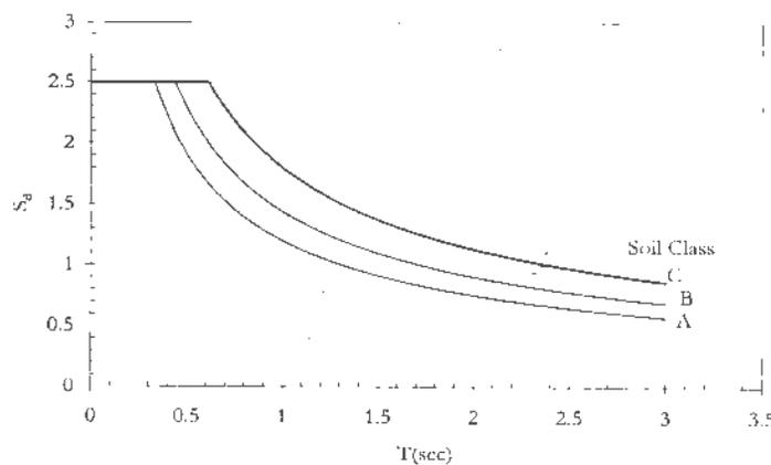
Figure 4: The design spectra of EBCS 8 for the ESF method of analysis for a bedrock acceleration ratio of,  $\alpha = 1$ , common occupancy structure ( $I=1$ ), and an elastic response of the structure ( $\gamma=1$ )
