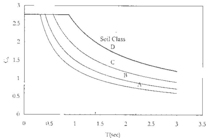
Figure 1 The design spectra of UBC 94 for  $I=1$ ,  $R_w=1$  and a base shear coefficient normalized with respect to the zone factor
