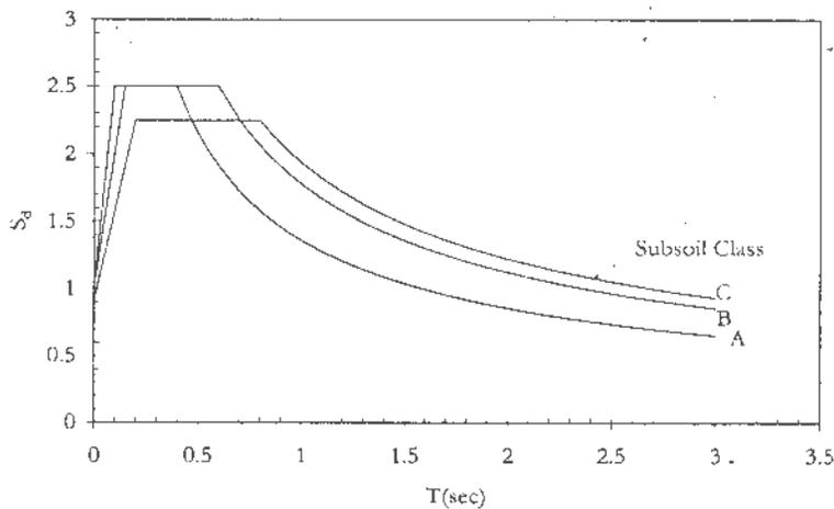
Figure 3 The design spectra of Eurocode 8 for the ESF method of analysis for a design ground acceleration ratio,  $\alpha = 1$ , and an elastic response of the structure ( $q=1$ )
