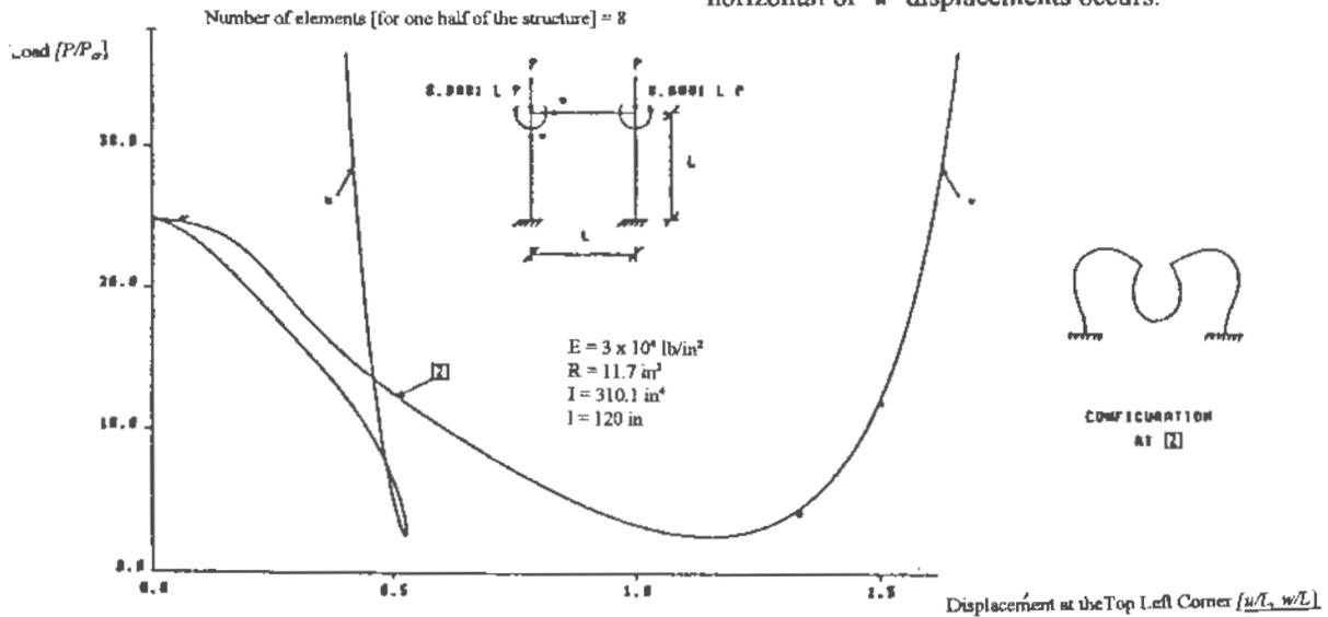
Figure 3 Plane load-displacement behavior of a fixed portal frame (symmetric mode)
