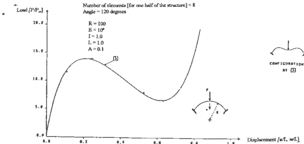
Figure 4 Plane load-displacement behavior of a fixed circular arch (symmetric mode)
