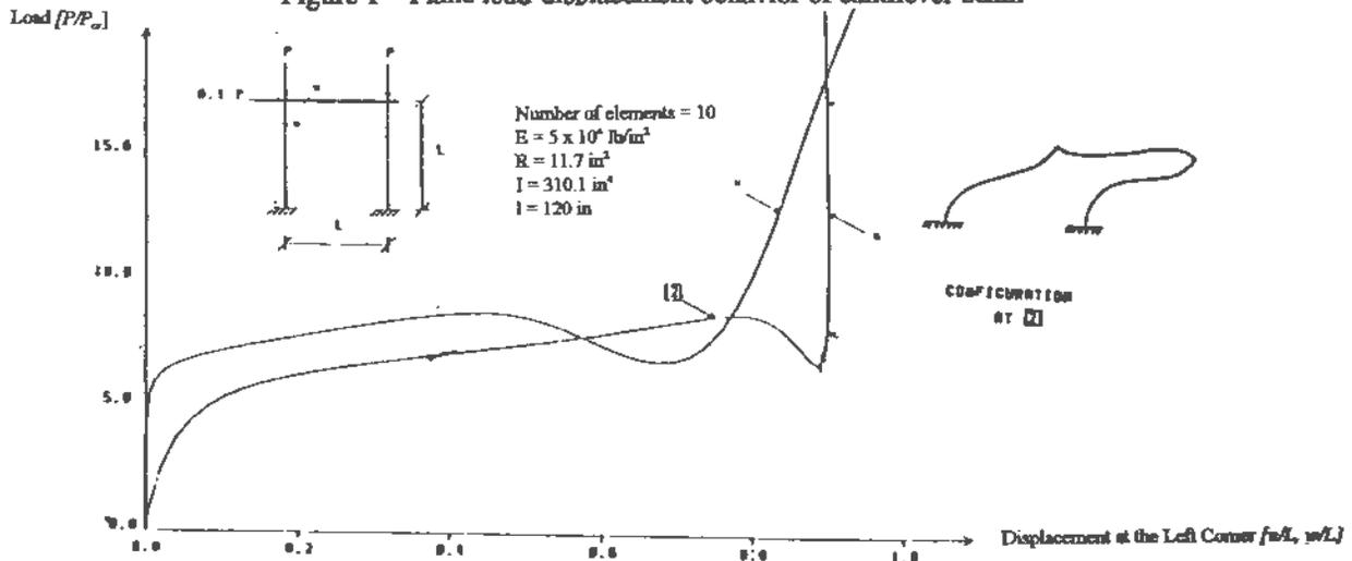
Figure 2 Plane load-displacement behavior of a fixed portal frame (unsymmetrical mode)
