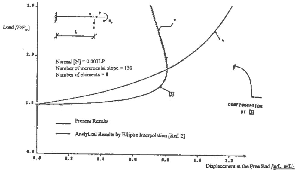
Figure 1 Plane load-displacement behavior of cantilever beam
