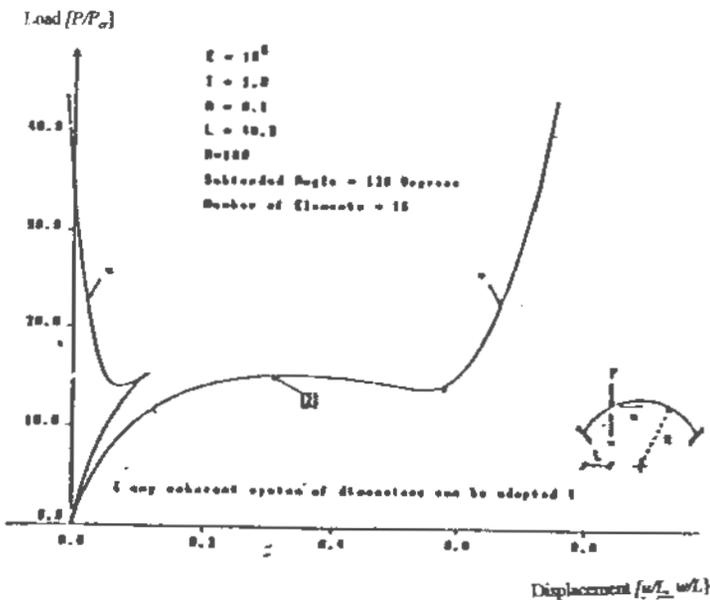
Figure 5 Plane load-displacement behavior of a fixed circular arch (unsymmetric mode)
