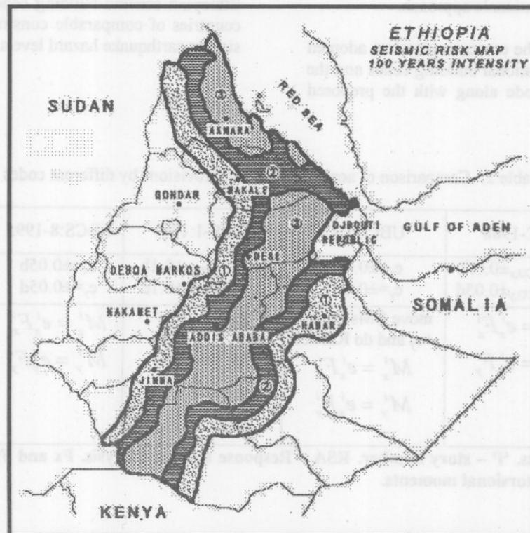
Figure 2 Seismic zoning of Ethiopia as per ESCP-1:1983
