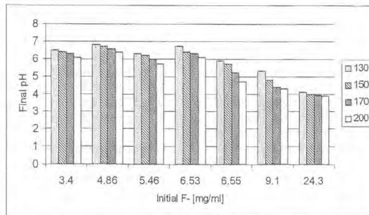
Figure 2 Dependence of Final  $pH$  on the initial fluoride conc. at different doses
