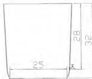
Figure 4 Final design for fluoride concentration of less than 10%, all units in cm.
