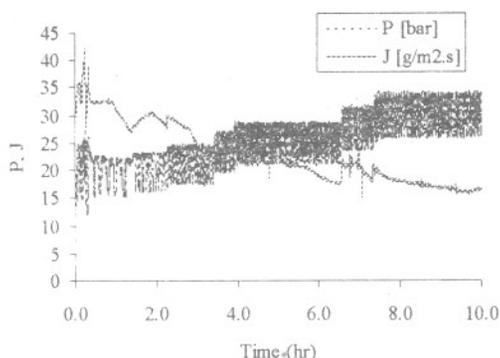
Figure 3. Pressure and flux vs. time during reverse osmosis of actual water from rift valley
