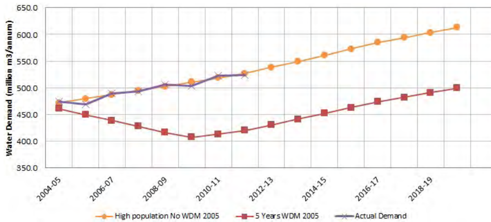
Figure 6 City of Johannesburg demand projection with and without WC/WDM versus actual demand
