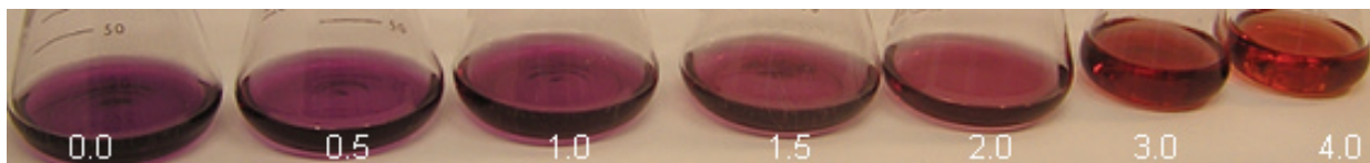
Figure 6 Reaction of fluoride in the range 0.0\text{--}4.0 \text{ mg}\cdot\text{l}^{-1} with 5 \times 10^{-5} M of aluminium chrome azurol B 1:2 complex
