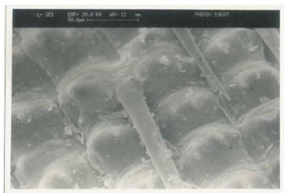
Figure 3 SEM photograph of outer surface of rice husk char (RHC)
