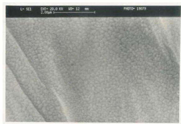
Figure 4 SEM photograph of inner surface of rice husk char (RHC)
