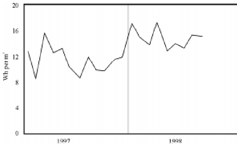
Figure 6 Energy efficiency at KWT Water Purification Works
