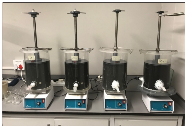
Figure 2. Augmented biosulphide potential (AugBSP) test equipment
