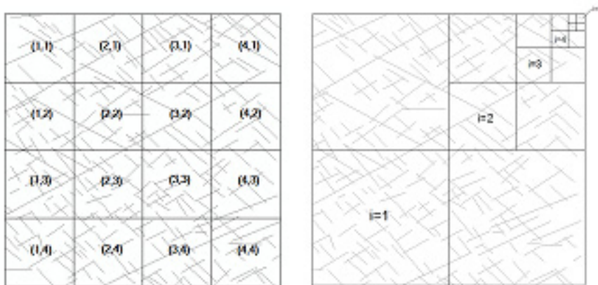
Figure 3 Equally spaced division of squared grid cells for segmenting lineaments—left: division controlled by row/column numbers; right: division by power number which automatically processes from bigger cells to smaller ones.
