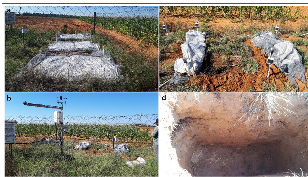
Figure 2. Experimental layout at the Bainsvlei site during the calibration process of DFM capacitance probes (a), soil, vegetation and slope characteristics at the plots were the same as for the existing ARC probe (b), 3 probes installed in a wet plot (c), 0.4 m wide and 0.8 m deep pit for bulk density sampling (d)
