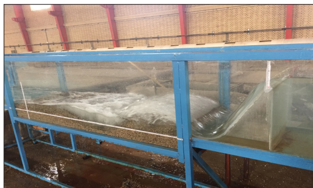
Figure 7. Impact of water jet with materials and formation of scour hole
