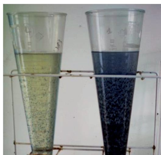
Figure 9. Real wastewater treated by Fenton process (left), by biological treatment (right) at the beginning of the sedimentation stage
