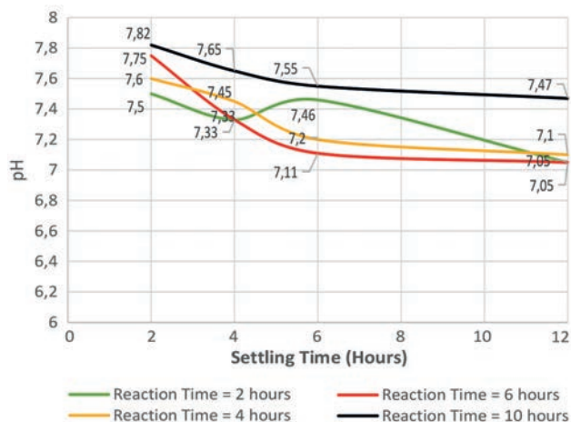
Figure 12 pH variation in CEPT-SBR system
