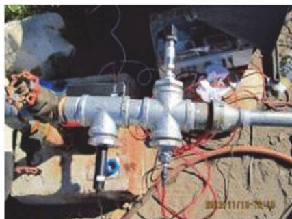
Figure 7 Borehole BH-1 and the set-up of the device for the aquifer test
