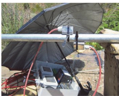
Figure 7 Borehole BH-1 and the set-up of the device for the aquifer test
