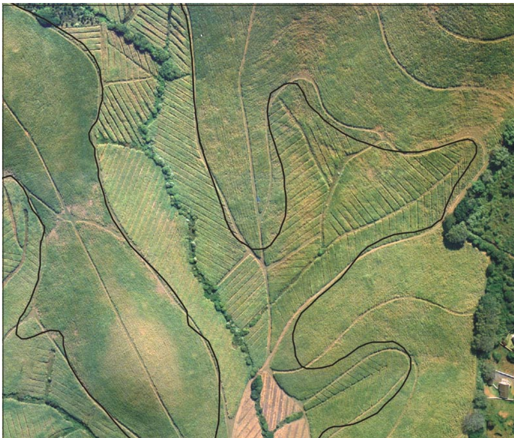
Figure 3 One of South Africa's 'lost' wetlands, the natural hydrological regime completely and permanently (but not necessarily irreparably) altered by an effective 'herringbone' network of drains, and natural hydrophytic vegetation replaced by sugarcane (wetland delineation detail undertaken by Land Resources International (Pty) Ltd., on behalf of Moreland Developments (Pty) Ltd.).
