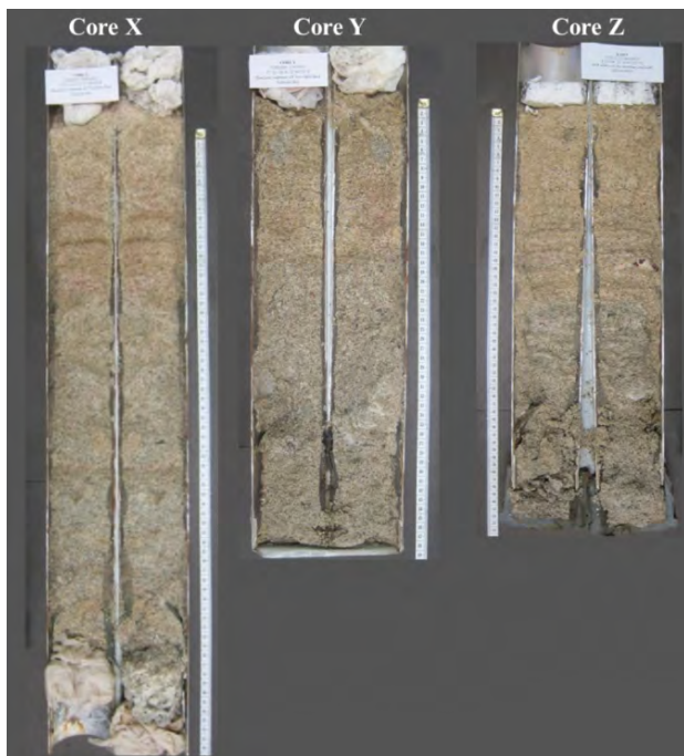
Figure 5. Sediment cores (X, Y and Z) collected inshore of Two-mile Reef. Bands common to all three cores are evident. The cores were 61, 49 and 47 cm in length, respectively; the scale bars are graduated in cm.
