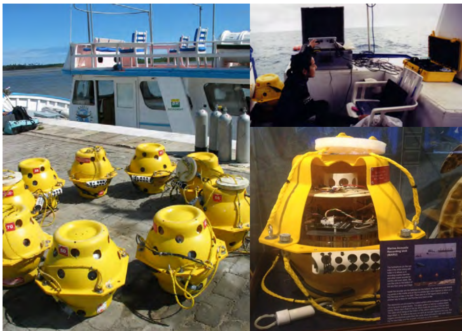
Figure 4. Array of marine autonomous recording units (MARUs) synchronized on land and tested before deployment. Photograph of a MARU showing the internal electronics and external hydrophone.
