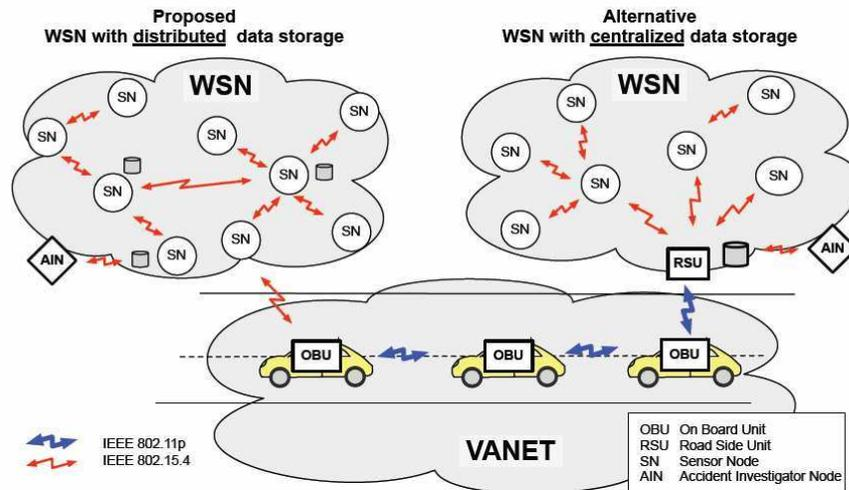
**Fig. 1.3: Systems architecture with distributed and centralized Data Storage[9][11]**
