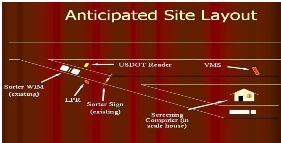
Figure 1.8: Proposed Roadside Vehicle identification layout [9].
