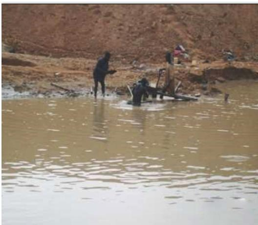
Fig. 3: The washing of sand from the Riverbed to trap alluvial gold at the Ankobra River, near Awudua Dada (Photo by D. Kumah, 2012)
