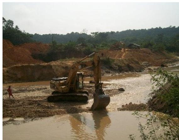
Fig. 6: Miners diverting the course of the river and scooping for alluvial gold (Photo by D. Kumah, 2012)
