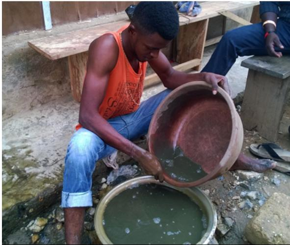
Fig. 14: Extracting gold from the “black” with the aid of mercury at Prestea
