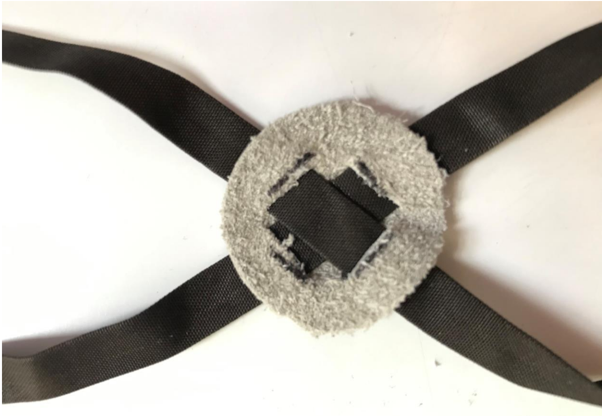
Figure 1.2: Teflon ribbon threaded through the slits cut in the soft leather-hub.
