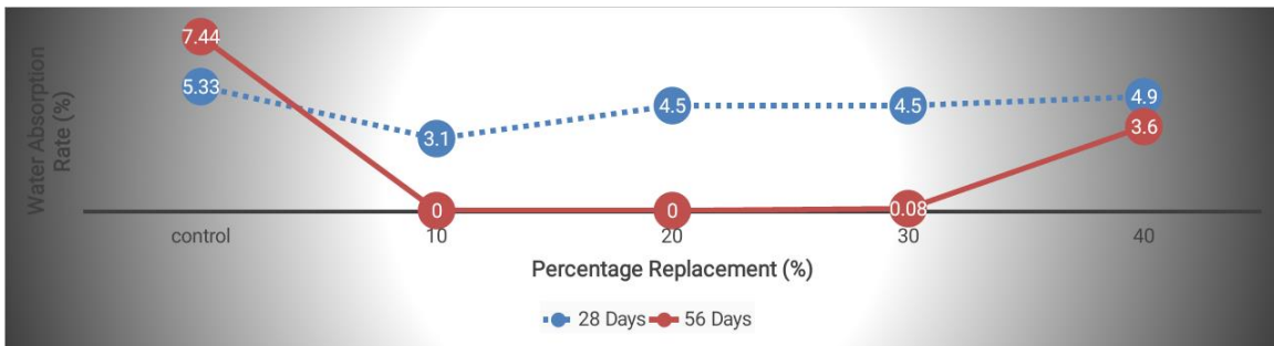
Fig. 9 Plot of Water Absorption Rate of 1000 °C Calcined Periwinkle Shell Ash on Laterized Concrete for Mix Ratio 1:1:2
