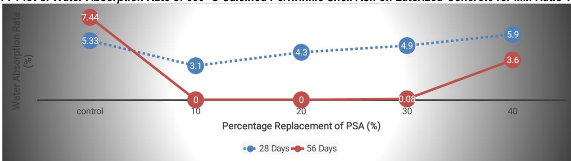
Fig. 8 Plot of Water Absorption Rate of 800 °C Calcined Periwinkle Shell Ash on Laterized Concrete for Mix Ratio 1:1:2
