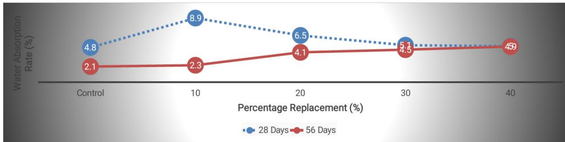
Fig. 11 Plot of Water Absorption Rate of 800 °C Calcined Periwinkle Shell Ash on Laterized Concrete for Mix Ratio 1:2:4
