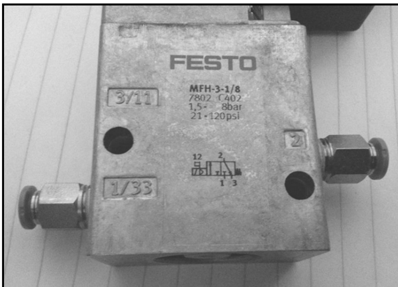
Figure 8: 3/2 way valve used as DCV
