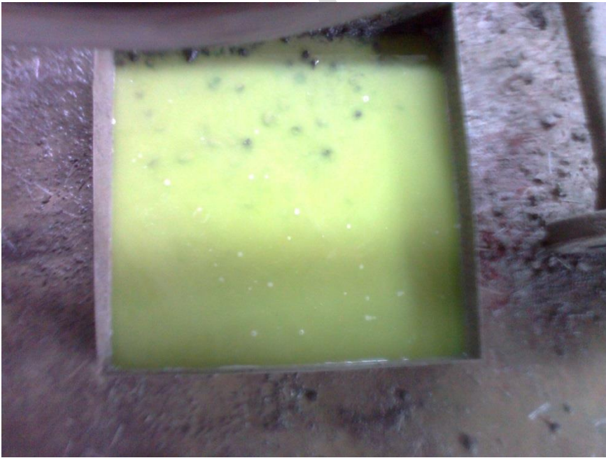
Figure 2: Green water due to tracer in the Penetron admix when added to concrete
