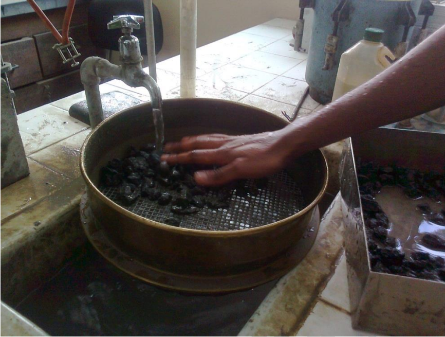
Figure 1: Washing of aggregates before preliminary testing
