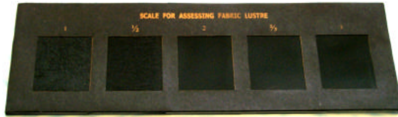
Figure 3.4 Physical Lustre Scale for the Subjective Assessment of Woven Fabric Lustre
