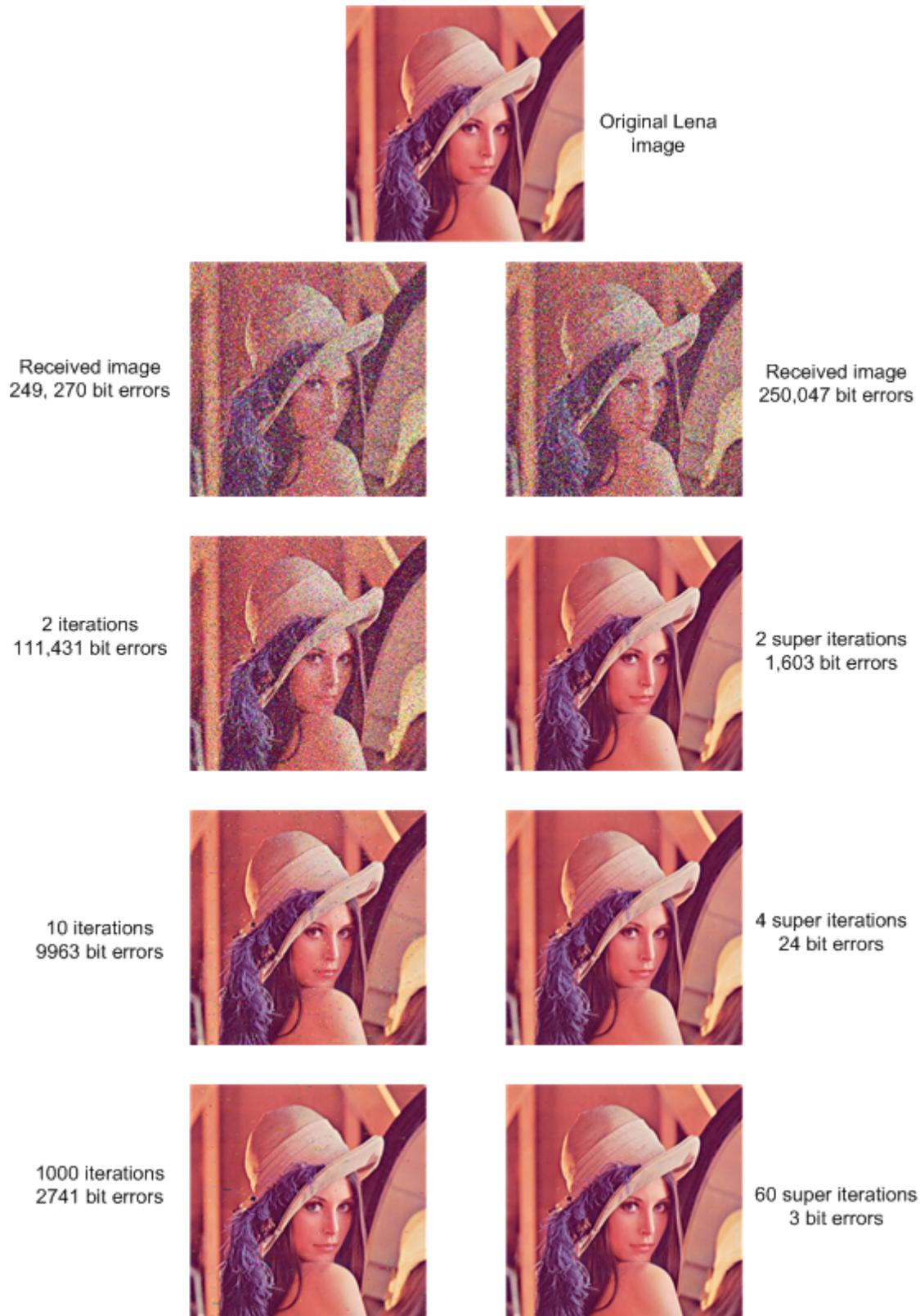
Figure 7: Performance of a TG code with  $k = 60$ ,  $n_1 = n_2 = 120$  with vs. a conventional LDPC code with  $k = 60$  and  $n = 240$  when applied to the decoding of a  $256 \times 256$  PPM lena image with 24 bits depth per pixel. Note that  $E_b/N_o = 3\text{dB}$ . The decoded images on the left column are LDPC decoded and those of the on the right column are TG decoded. Notice the large difference in bit errors of the two schemes.
