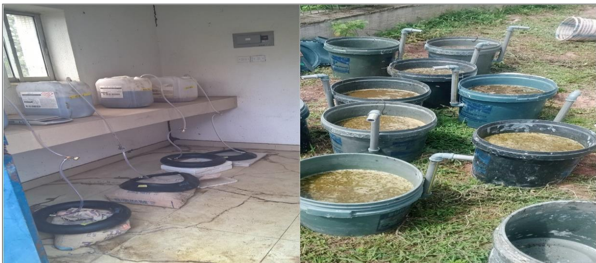
Figure 5: Locally fabricated digesters and slurry preparation process
