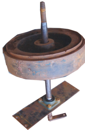
Figure 8. Assembled industrial bearings, shaft, fly wheel and connecting pan.
