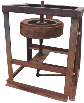
Figure 9. The fly wheel, shaft, industrial bearing and connecting rod fixed on the frame.
