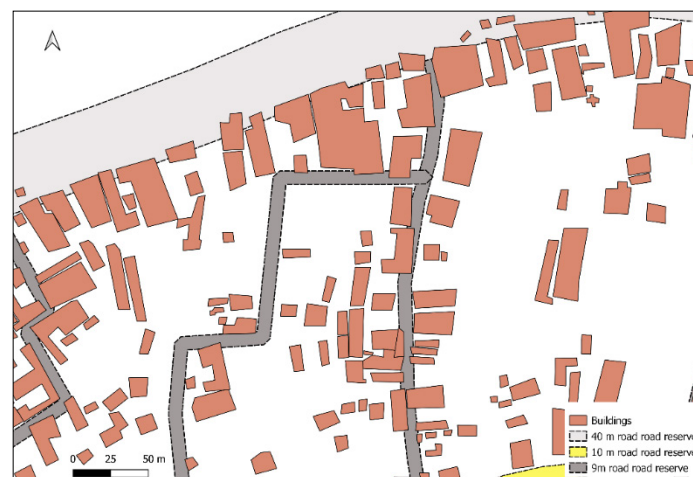
Figure 3: Overlay of buildings and road reserves (note the buildings encroaching on road reserves)
