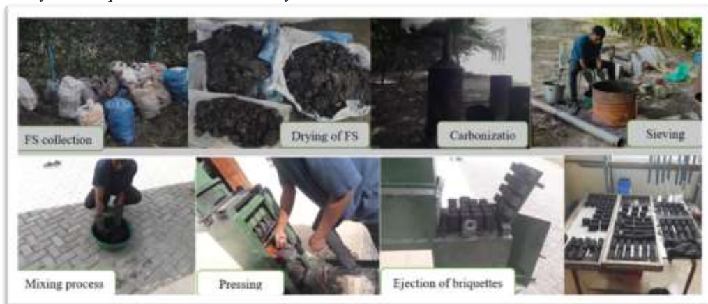
Figure 2: Practical procedures for briquettes production
