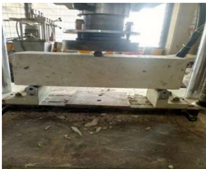
Figure 14: Three-point flexural strength test
