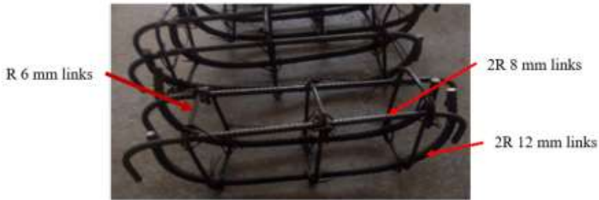
Figure 6: Fabricated steel cages/bars used in the study
