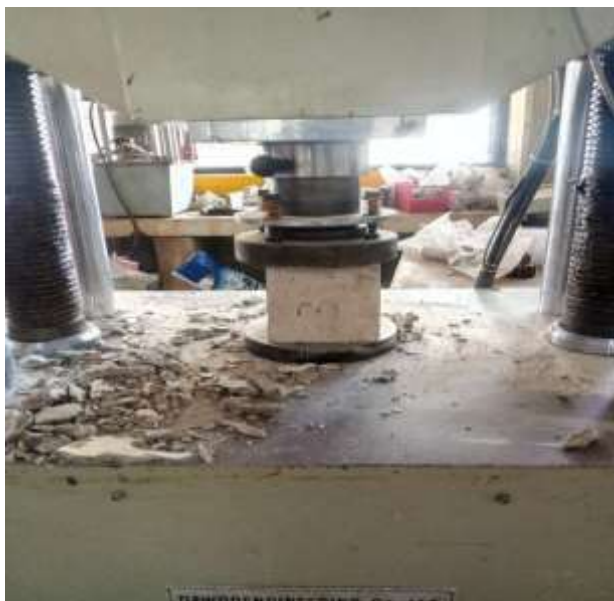
Figure 11: Compressive Strength Testing
