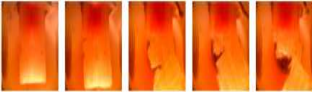
Figure 7: Images showing evolution of the choke valve probe due to erosion.
