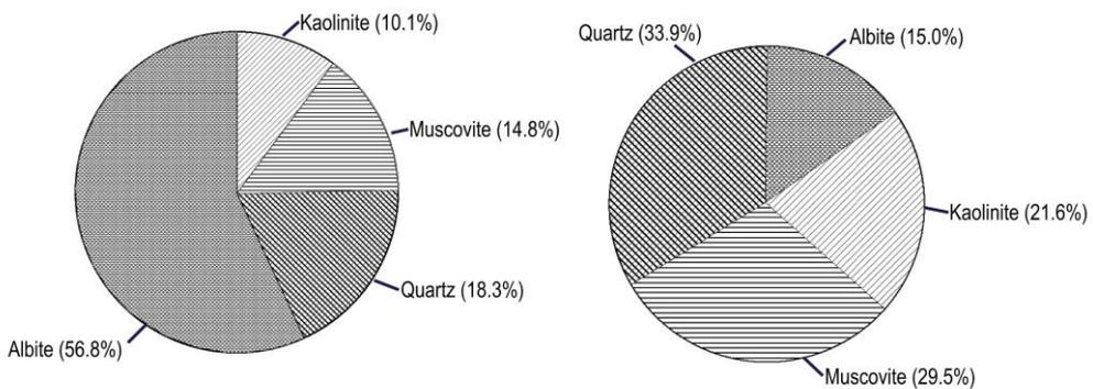
**Figure 3:** Phase composition (wt%) of the two representative samples calculated by the Reference Intensity Ratio (RIR) method showing the amount of kaolinite, albite, quartz and muscovite.
