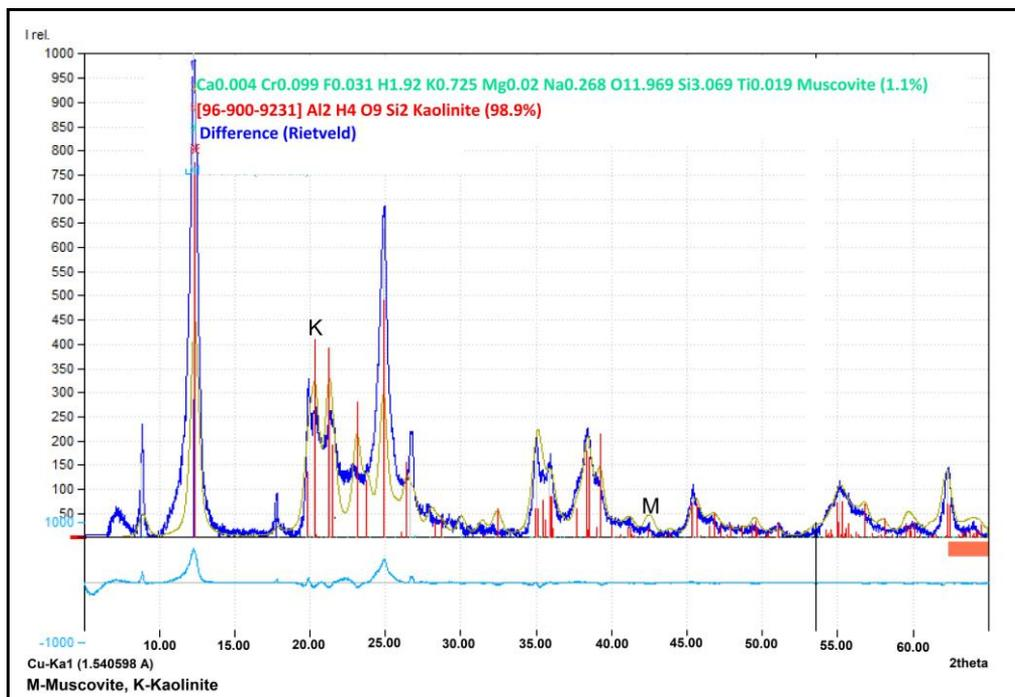
**Figure 4:** Representative X-ray diffractogram of the kaolin from the Matamba deposit showing kaolinite and muscovite minerals.
