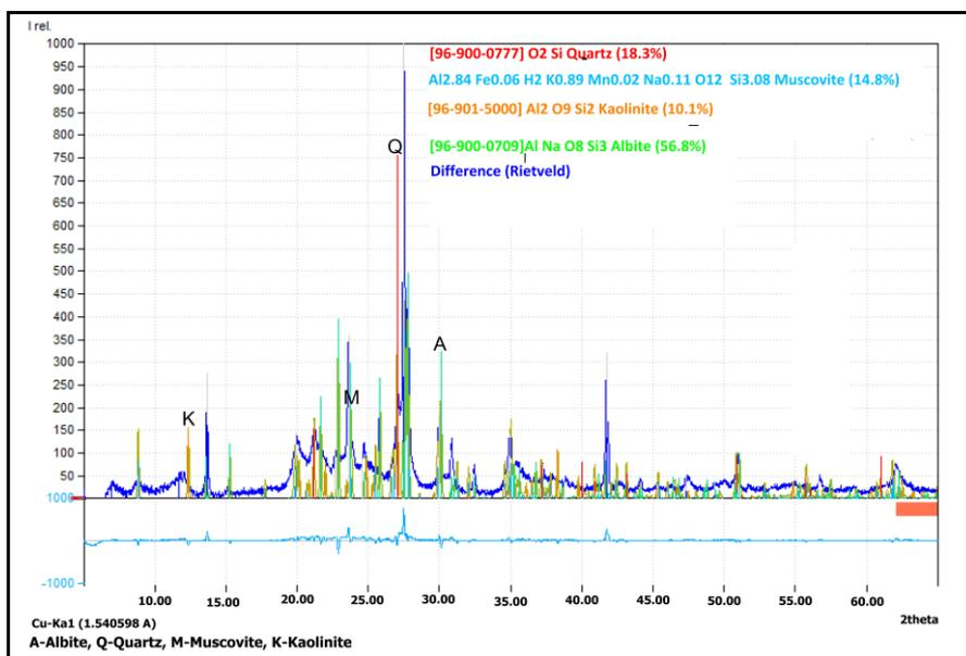
**Figure 6:** Representative X-ray diffractogram of the kaolin from the Matamba deposit showing kaolinite, albite, quartz and muscovite minerals.
