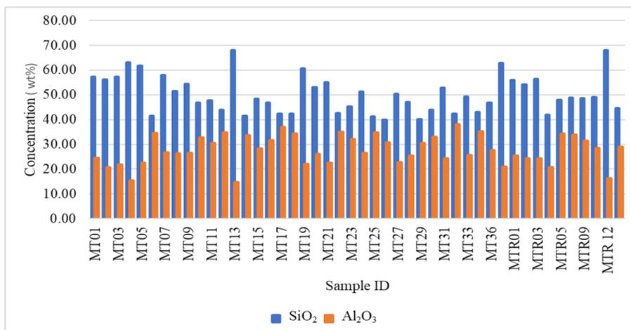
**Figure 72:** A bar chart of SiO<sub>2</sub> and Al<sub>2</sub>O<sub>3</sub> concentration (wt%) of the representative samples from the Matamba kaolin deposit.
