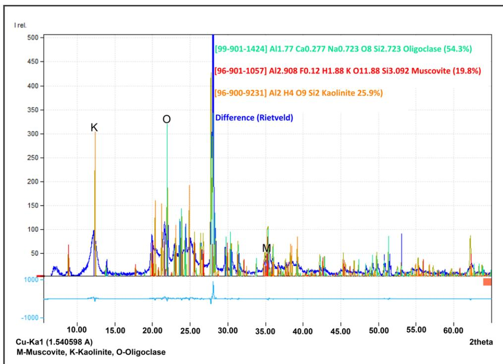
**Figure 5:** Representative X-ray diffractogram of the kaolin from the Matamba deposit showing kaolinite, oligoclase and muscovite minerals.
