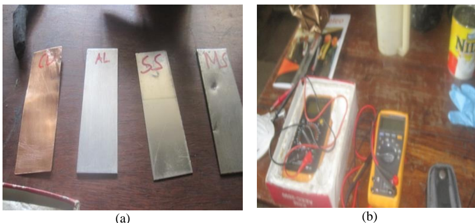
Figure 2: Photos of (a) electrode materials: CU-copper, AL-aluminium, SS-stainless steel, and MS-mild steel; and (b) digital multimetres.
