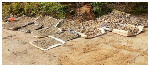
Plate 1: Samples of clay and granite dust being sun dried.
