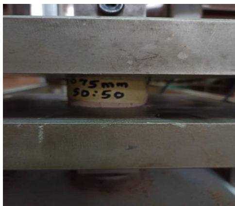
Plate 4: Compression strength samples under test.
