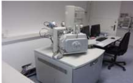
Figure 3: MLA 650 FEI system set up for mineral liberation studies.
