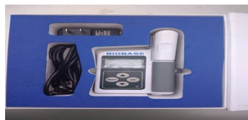
Figure 2: Portable chlorophyll meter, product model; CM-8, serial number: TP201933112103 Electric supply; 220V 50Mz.
